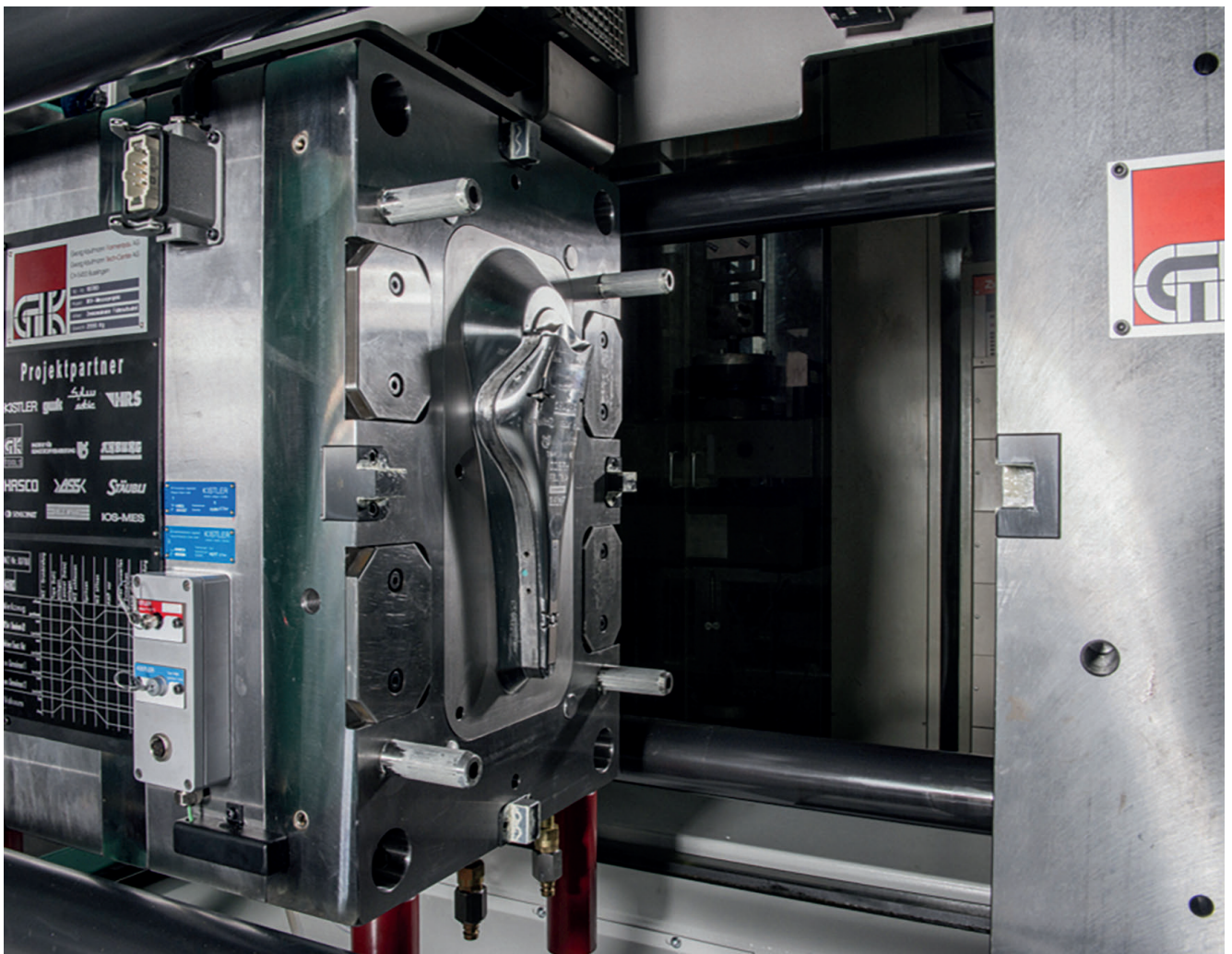
The experimental mold with the cavity of a bicycle saddle has a servo-electrically driven hot runner © IKV
